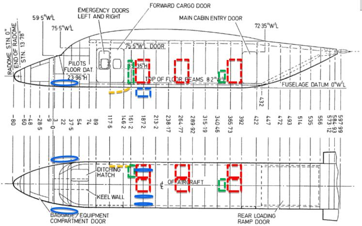
**Schematic of a notional layout** of the SAM-CAAM Payload Option C in the NASA C-23B Sherpa aircraft. Two-bay racks are shown in red, in-cabin floor-mounted instruments in green, external probes in blue, and the aerosol inlet in gold. The point of this notional payload is to demonstrate *feasibility*.
