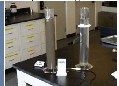
Soil Hydrometer apparatus
