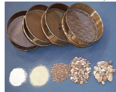
Sieves for mechanical analysis
