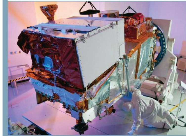
Figure 1. High level VIIRS Flight Unit 1 and Flight Unit 2 instrument characteristics with photo of FU1 being integrated onto the NPP spacecraft at Ball Aerospace. Photo courtesy Ball Aerospace.
